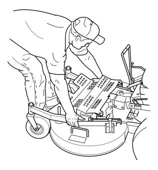
Figure 4-17 Removing The Deck
